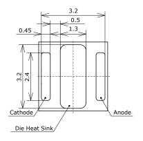
Figure 2. Electrode Configuration
